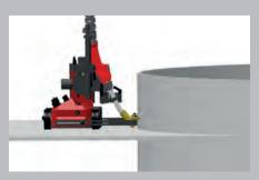
/ Welding fillet welds on convex components
