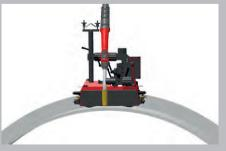
/ Welding butt welds on convex components
