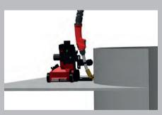
/ Welding fillet welds on convex components
